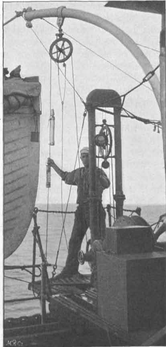
Lotmaschine System Sigsbee.
