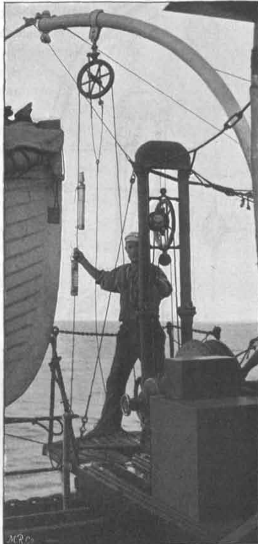
Lotmaschine System Sigsbee.
